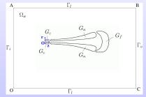
A penalization method to take the net and fishes into account : Navier-Stokes/Brinkman model with eddy viscosity ⇒ Possibility of 3D computations by the means of a Fighting Domain Method and complex methods.
