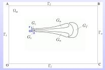
A penalization method to take the net and fishes into account : Navier-Stokes/Brinkman model with eddy viscosity ⇒ Possibility of 3D computations by the means of a Fictitious Domain Method : no complex mesh
