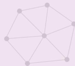
Zienkiewicz-Zhu (ZZ) error estimator  $\int_K \left( \frac{\partial e}{\partial x_1} \right)^2 \rightarrow \int_K \left( \frac{\partial u_h}{\partial x_1} - \Pi \frac{\partial u_h}{\partial x_1} \right)^2$
